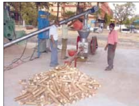
Fig. 2. Binderless briquetting of crop residues
