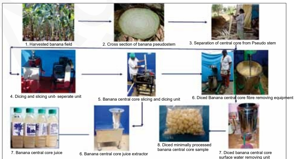
Fig. 7. Mechanization package for minimal processing and juice extraction from banana central core.
