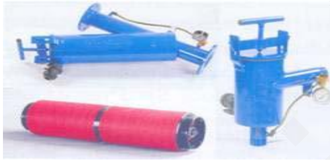
Fig.1.5 Disk filter showing stacks of discs
