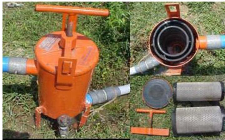
Fig.1.3 Screen filter showing steel wire mesh strainers
