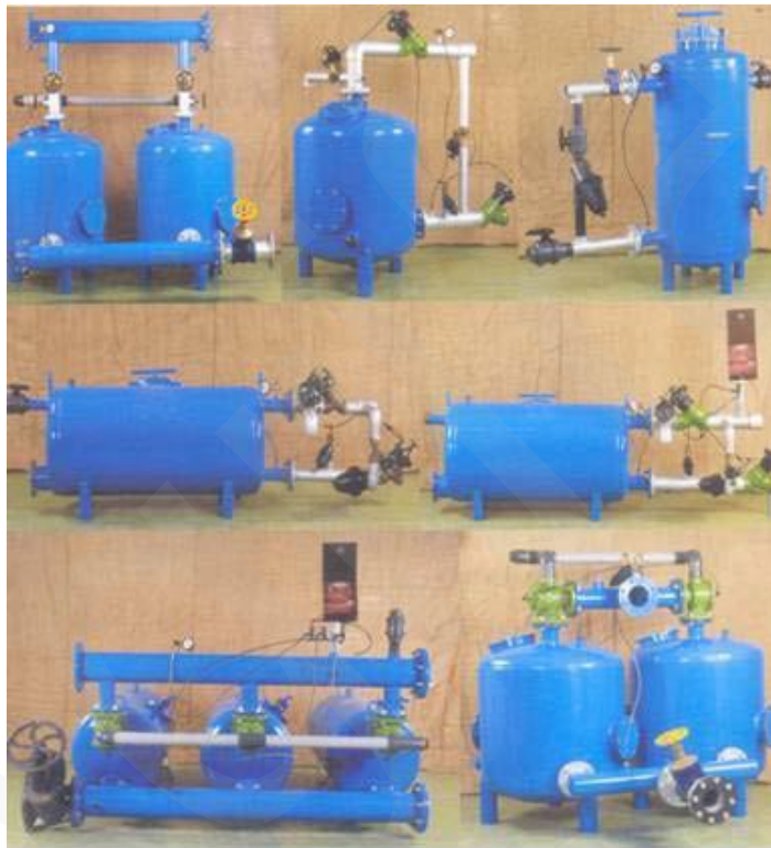
Fig. 1.2 Different types of Media filters
